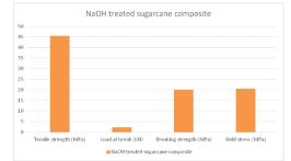
Figure.9. Tensile properties of NaOH treated sugarcane bagasse composite
